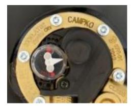
**5** Safety valve - if the gas pressure inside the refillable gas bottle exceeds 27 bar, the safety valve blows off gas in a controlled manner to prevent the refillable gas bottle from bursting.
